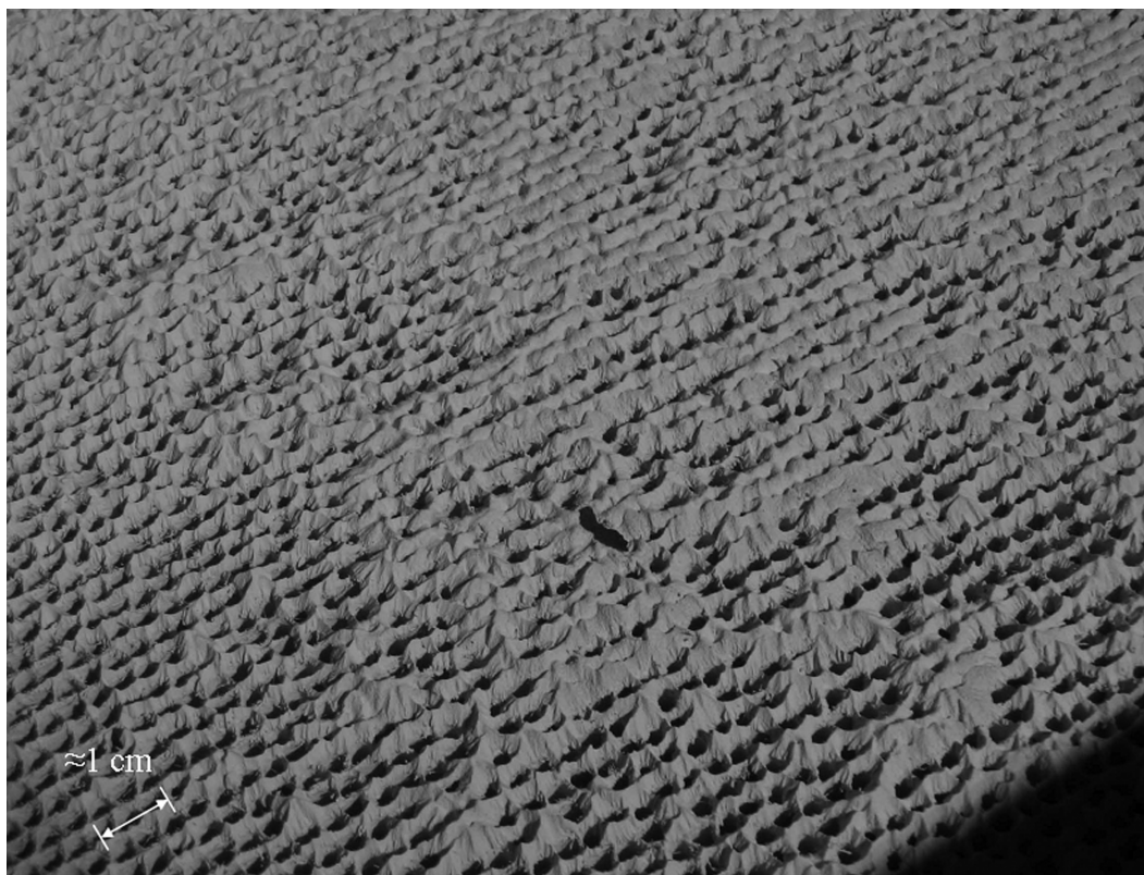
Figure 1. Example of particle deposition in the SCR reactor in the low dust position of a waste incineration plant after 15,000–20,000 h of operation.
